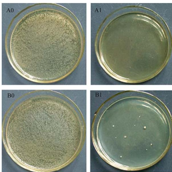
**Fig. 1** The breeding status of *E. coli* on the samples: CNTs sample without Cu coating (A0); pyrolytic carbon without Cu coating (B0); CNTs sample with Cu coating (A1); pyrolytic carbon with Cu coating (B1)
