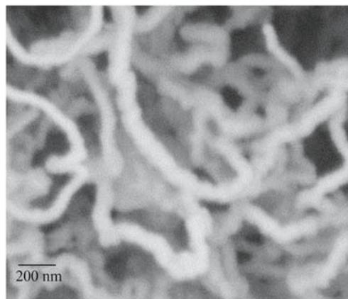
**Fig. 4** SEM image of Cu coated CNTs sample (A1)
