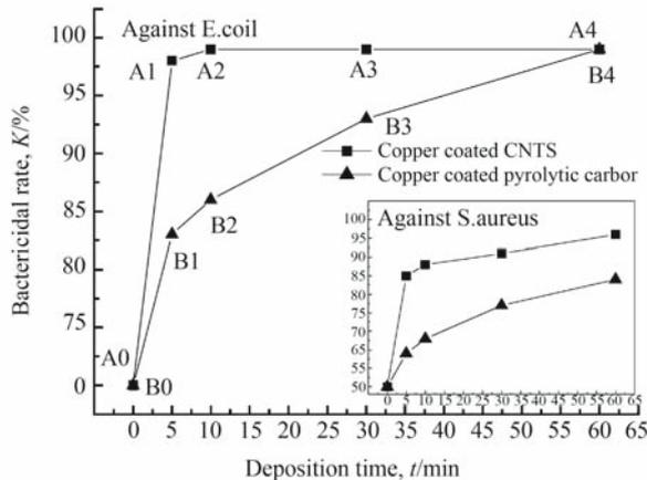
**Fig. 2** The bactericidal rate of Cu coated CNTs samples and Cu coated pyrolytic carbon samples
