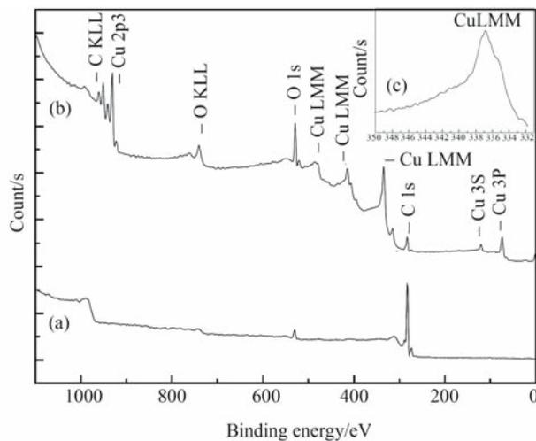
**Fig. 3** (a) XPS spectrum of CNTs sample A0; (b) XPS spectrum of Cu coated CNTs sample A1; (c) Cu LMM XPS spectrum for Cu coated CNTs sample A1
