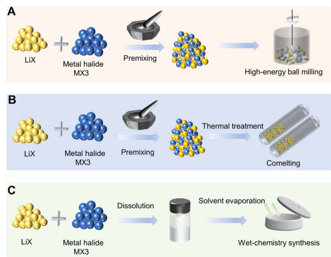
Fig. 4. Synthesis methods of halide SSEs. (A) High-energy ball milling. (B) Comelting. (C) Wet-chemistry synthesis.
