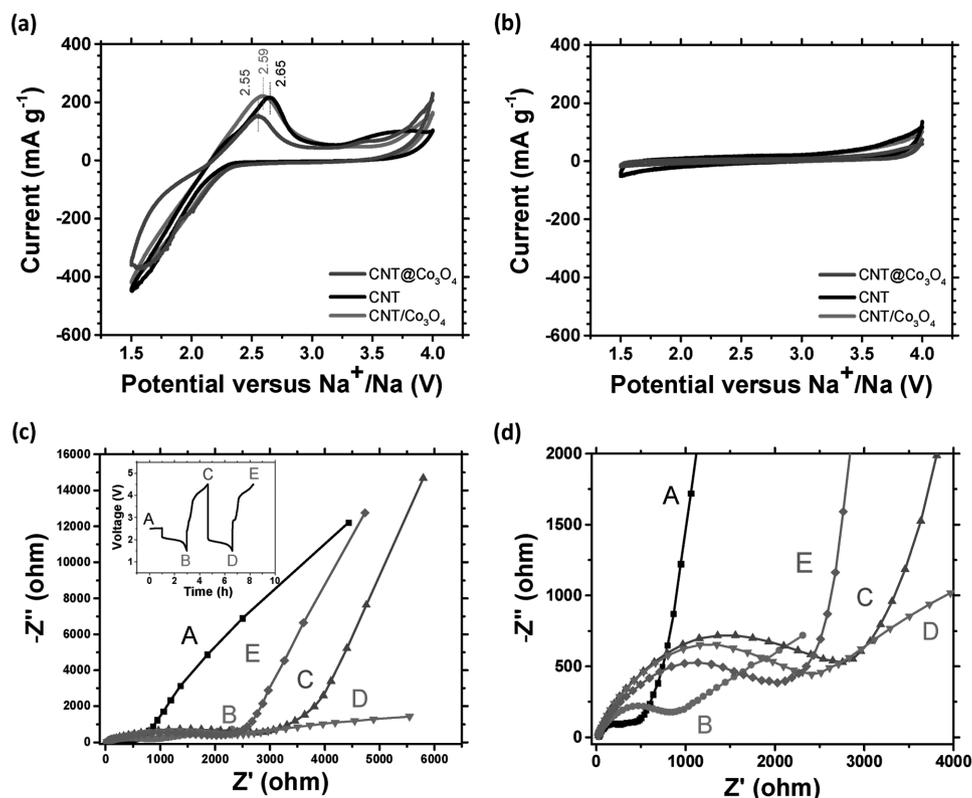
**Figure 4.** CVs of ALD CNT@Co<sub>3</sub>O<sub>4</sub>, CNT/Co<sub>3</sub>O<sub>4</sub> nanocomposite air electrodes, and pristine CNT under a) dried air and b) Ar. c,d) EIS spectra of SABs with ALD CNT@Co<sub>3</sub>O<sub>4</sub> at initial, 1st, and 2nd discharged/charged states at a current density of 300 mA g<sup>-1</sup>; inset of (c) shows the charge and discharge curves showing the state of charge/discharge for collecting EIS; (d) shows the low frequency region of (c).
