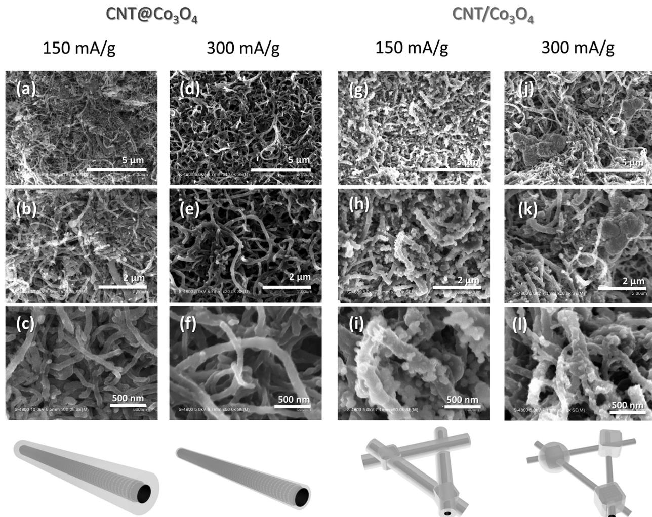
**Figure 6.** Morphology of discharged a–f) ALD CNT@Co<sub>3</sub>O<sub>4</sub> and g–l) CNT/Co<sub>3</sub>O<sub>4</sub> nanocomposite air electrodes at the current densities of 150 and 300 mA g<sup>-1</sup>. Schematic graphs are also shown.
