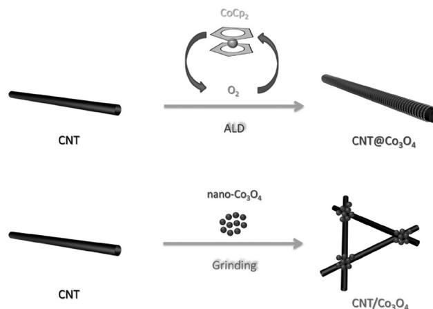
**Figure 1.** Schematic diagram of the fabrication of ALD CNT@Co<sub>3</sub>O<sub>4</sub> and mechanically grinded CNT@Co<sub>3</sub>O<sub>4</sub> nanocomposite.
