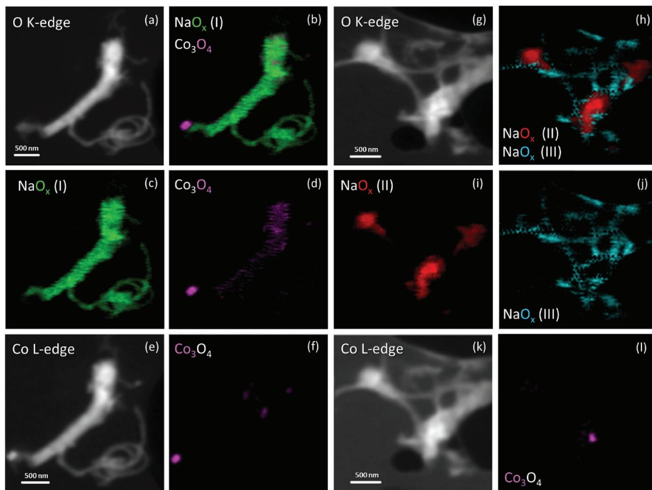
**Figure 9.** a,g) O K-edge and e,k) Co L-edge optical density images (average stacks) of discharged ALD CNT@Co<sub>3</sub>O<sub>4</sub> and g–l) CNT/Co<sub>3</sub>O<sub>4</sub> nanocomposite air electrodes. STXM chemical imaging of discharged b–d, f) ALD CNT@Co<sub>3</sub>O<sub>4</sub> and h–j, l) CNT/Co<sub>3</sub>O<sub>4</sub> nanocomposite air electrodes by extracting XANES spectra of Co<sub>3</sub>O<sub>4</sub> and different types of NaO<sub>2</sub>.
