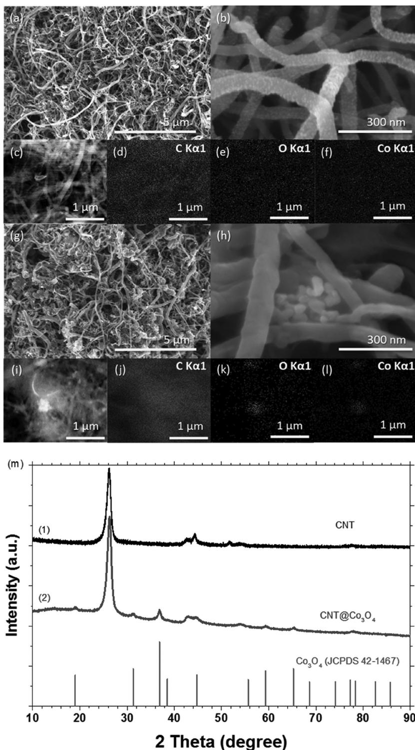
**Figure 2.** Morphology and element distribution of a–f) ALD CNT@Co<sub>3</sub>O<sub>4</sub> and g–l) CNT/Co<sub>3</sub>O<sub>4</sub> nanocomposite by SEM and EDX mapping. m) XRD pattern of (1) pristine CNT and (2) ALD CNT@Co<sub>3</sub>O<sub>4</sub>; standard XRD pattern of Co<sub>3</sub>O<sub>4</sub> from JCPDS database is also shown for comparison.
