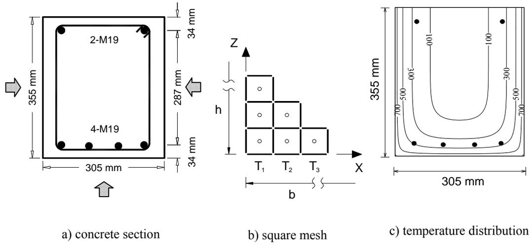
Figure 2. Heat transfer analysis of a concrete beam exposed to fire from three sides.
