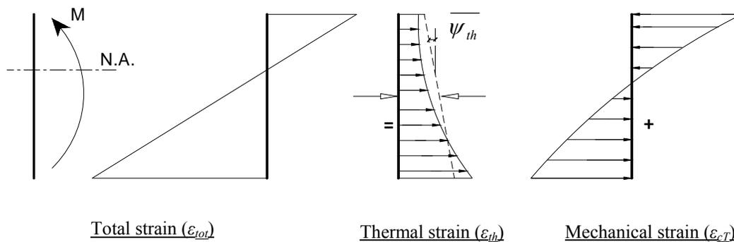
Figure 4. Components of total strain at elevated temperatures.
