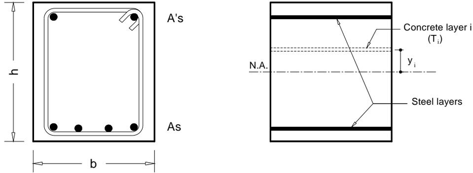
Figure 1. Cross-section and fiber model of the analyzed RC beam.
