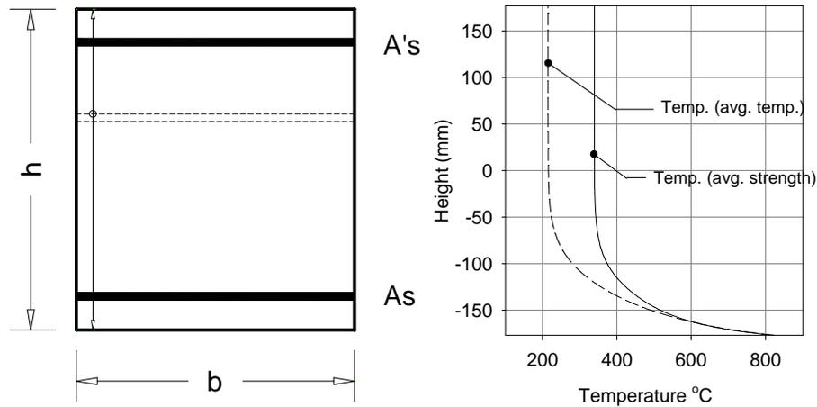
Figure 3. Average temperature distributions for beams during fire exposure.
