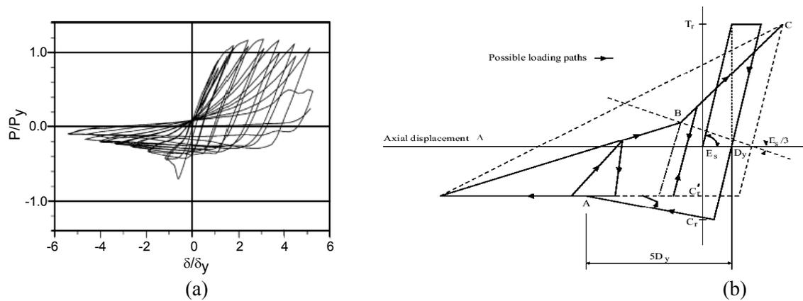
Figure 6. (a) Typical hysteresis of a steel bracing member under cyclic load (Tremblay 2002); (b) Model hysteresis of steel brace proposed by Jain and Goel (1978)
