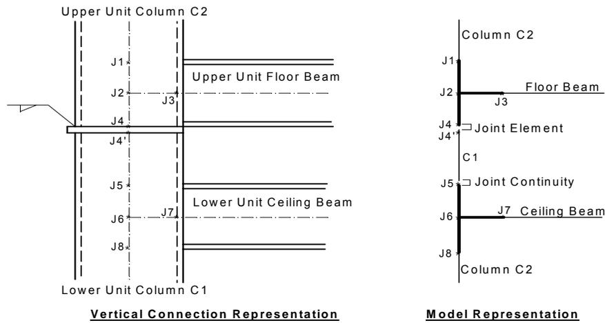
Figure 5. Model of vertical connection of units of MSB braced frame
