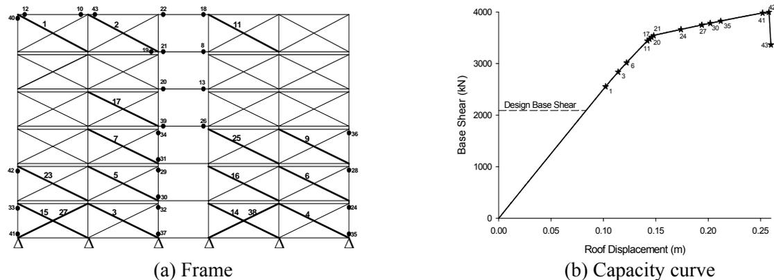
Figure 7. Sequence of yielding/buckling of the 6-storey MSB braced frame (brace induced column actions by SRSS accumulation approach)
