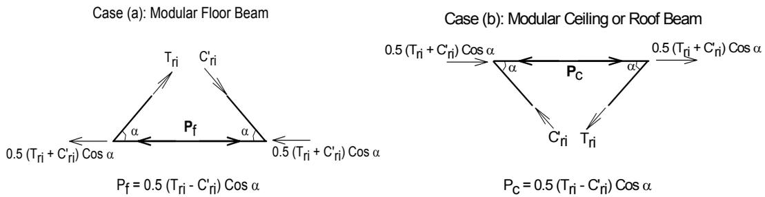
Figure 4b. Free body diagrams of beam forces to support redistributed brace loads
