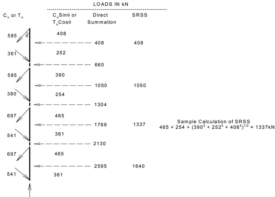
Figure 4a. Cumulative brace loads for determining column actions in 4-story MSB
