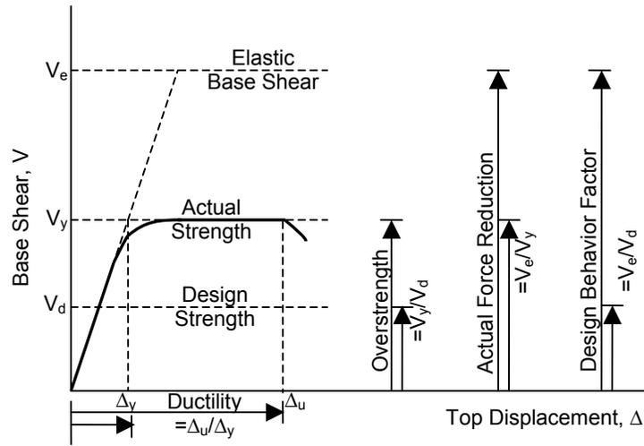
Figure 1. Typical structural response envelope
