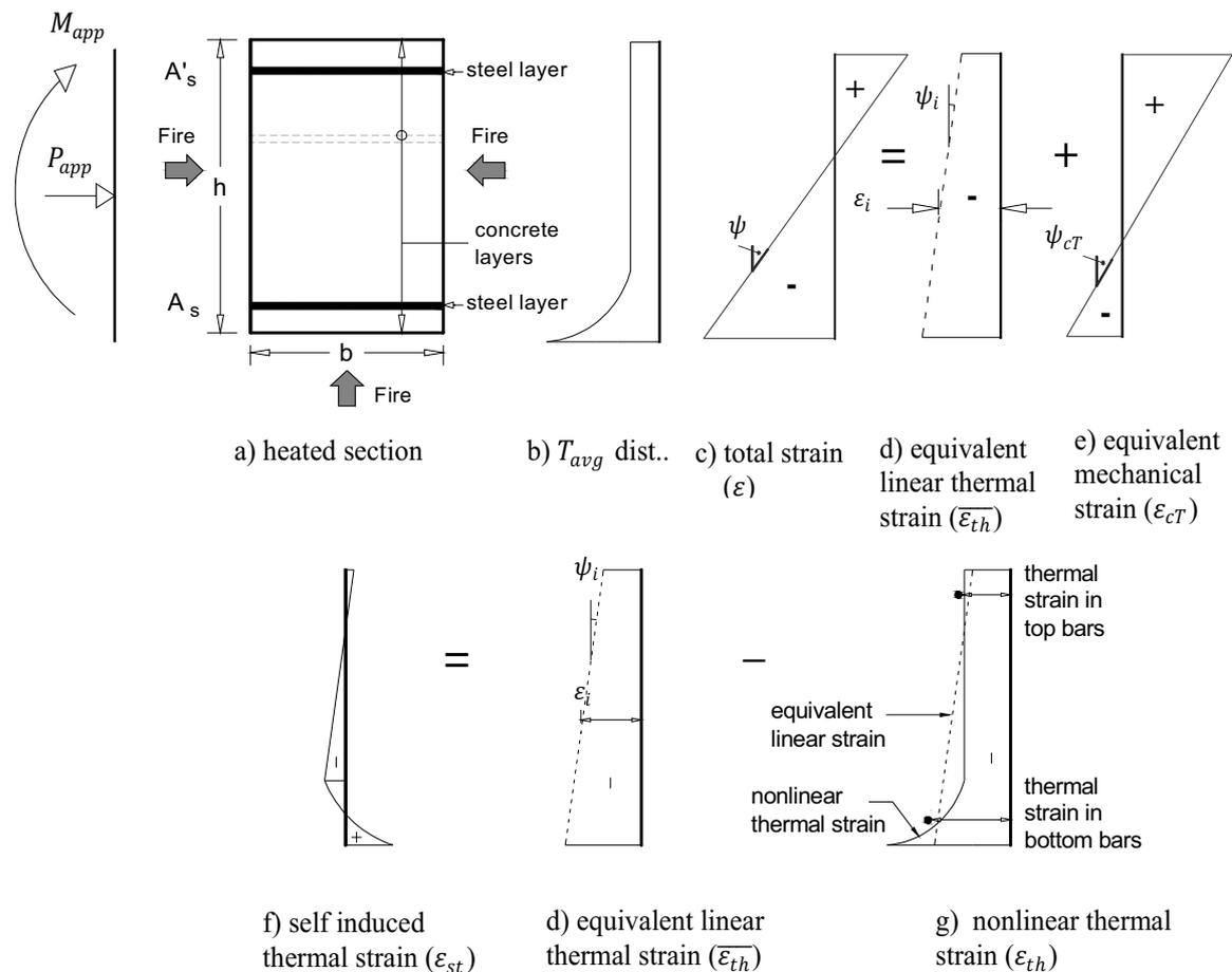
Fig. 1 Sectional analysis approach for heated RC sections
