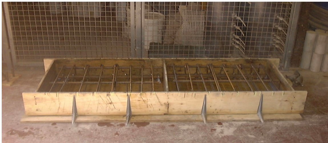
Figure 2 Two Reinforced Concrete Specimens
