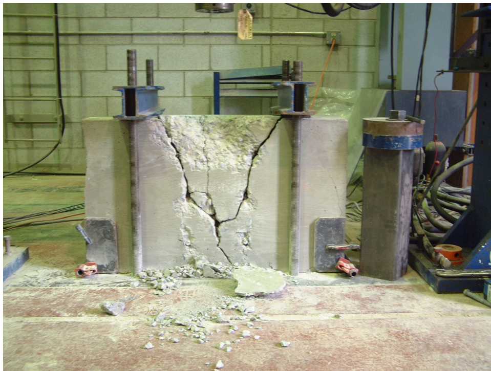
Figure 16 Shear Failure of Plain Concrete Block (Tests V3 and V4)
