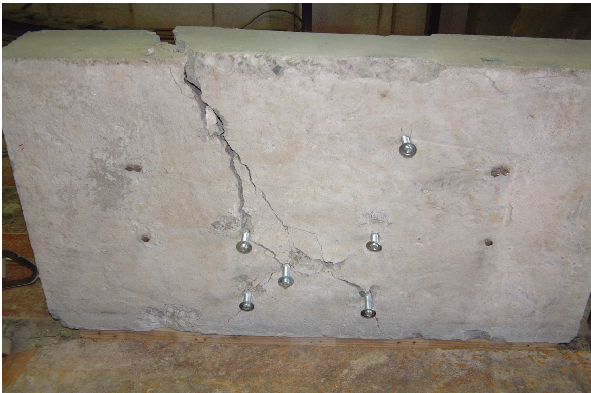
Figure 12 Shear Failure of Plain Concrete Block (Test V2)
