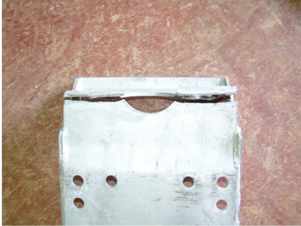
Figure 21 Failed Uplift Bracket during Tests V6 and V7
