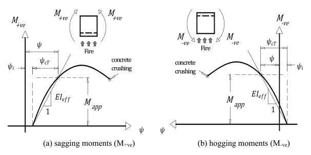
Fig. 2 (M)– $(\psi)$  diagrams for RC sections during fire
