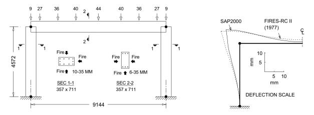
Fig. 3 Layout for a RC frame exposed to ASTM-E119 fire [Dims in *mm*, loads in *kN*]
