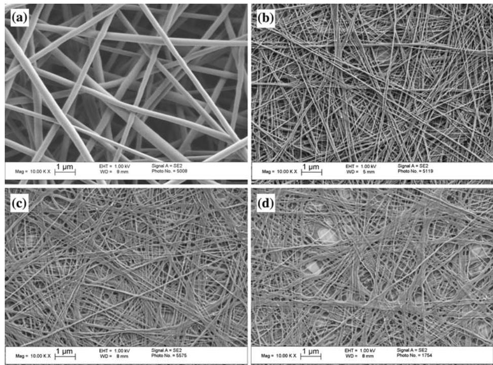
**Fig. 3** SEM images of PVA fibers with 4 h of 110 °C annealing treatment after **a** annealing, **b** immersed in DI water for 1 day, **c** immersed in DI water for 10 days, and **d** immersed in DI water for 30 days
