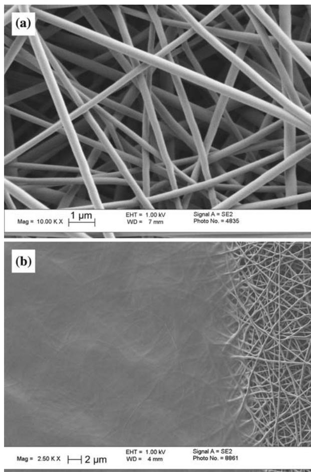
**Fig. 1** SEM images of original PVA fibers **a** in high magnification and **b** after immersed in DI water for 1 min (area affected at the left side)
