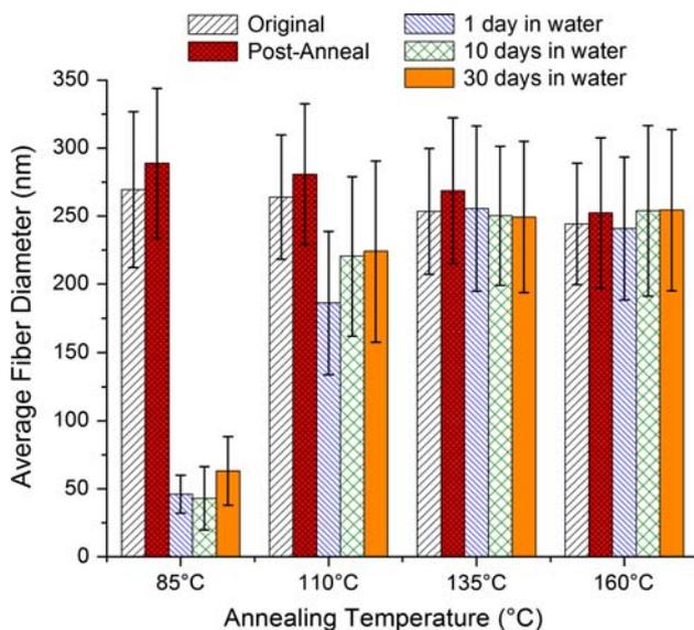
**Fig. 6** Fiber diameters after 4 h of annealing at four different temperatures; at five different stages during the stability test in DI water (the error bars are standard deviation)
