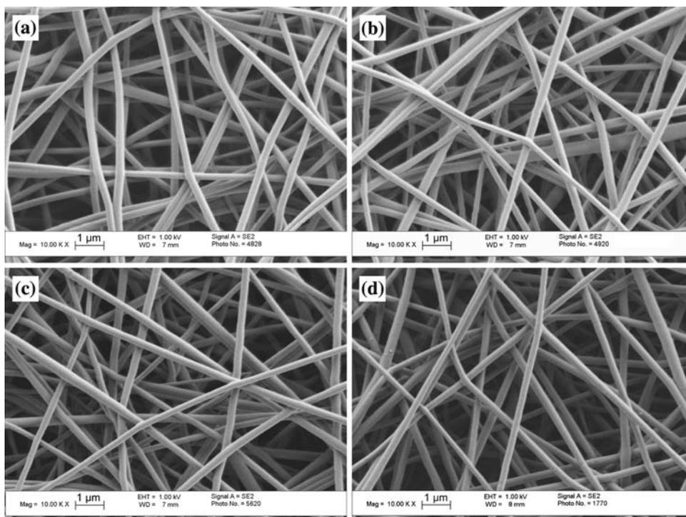
**Fig. 5** SEM images of PVA fibers with 4 h of 160 °C annealing treatment after **a** annealing, **b** immersed in DI water for 1 day, **c** immersed in DI water for 10 days, and **d** immersed in DI water for 30 day
