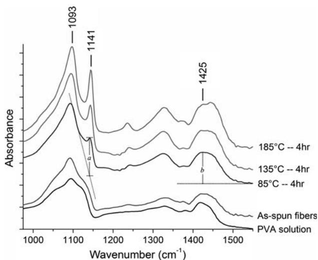
**Fig. 10** FTIR spectra (in the range between 975 and 1550  $\text{cm}^{-1}$ ) of PVA solution, as-spun fibers, and fibers after 4 h of 85 °C annealing, 4 h of 135 °C annealing and 4 h of 185 °C annealing (arbitrary scale on absorbance intensity and offset for clarity)
